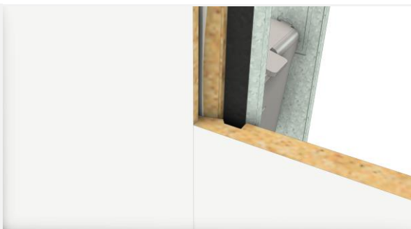
The silicone glue holds the connection in place.
