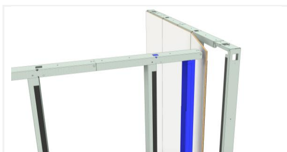
Mount the panels to the 1 st structure.
