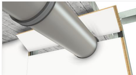
Put in place the top piece of the panel.
