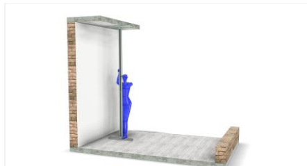
Clamp the module between the floor and ceiling by closing the Quicksan. Fasten the module in place like in chapter 3.4.
