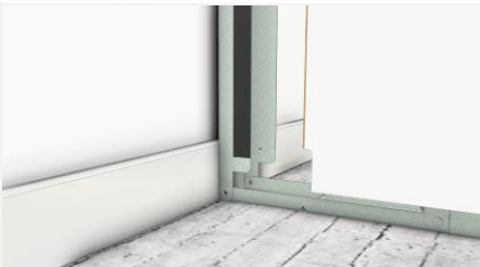
Make a cut-out in the click panel for the skirting board.
