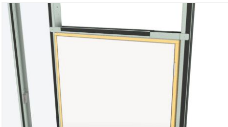
Place the header on the frame and slide it open. No need to screw it on.
