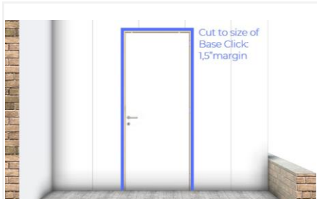
If the door frame has an architrave, the click panels do not have to be perfectly aligned with the frame. A margin of 1.5" is possible. In any case, ensure that the panels do not touch the door frame so that acoustic leak is avoided.
