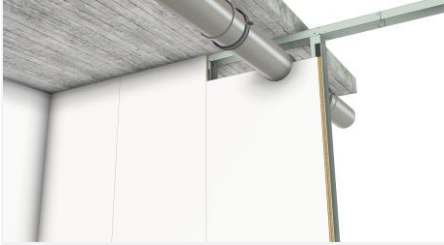
Without the pipe, the panel could rotate to snap into the 2 nd panel. The pipe prevents this movement.
