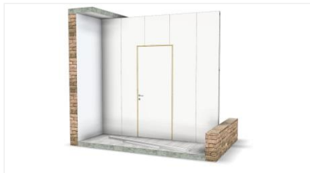
Attach the click panels to the modules.
