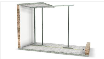
Insert the I-modules. Insert a door top profile in the place of the door opening.
