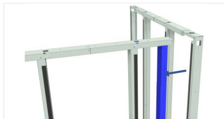
Position the angled structure, but do not fix the adjacent C-module (blue) yet; slide it into the left.
