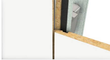
The cut groove allows the tongue of the 3 rd panel to slide sideways into the 2 nd panel. This requires a 3 mm clearance around the pipe itself.
