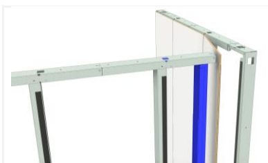
Mount the panels to the 1 st structure.
